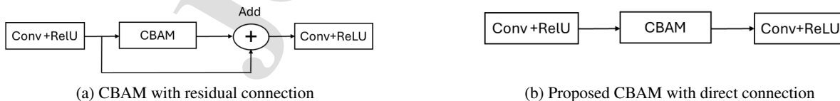
Figure 2: CBAM integration strategies: (a) the original design employing a residual connection between the input feature map and the CBAM output, and (b) the proposed variant that directly feeds the CBAM output into the subsequent convolutional operation without a residual connection.
